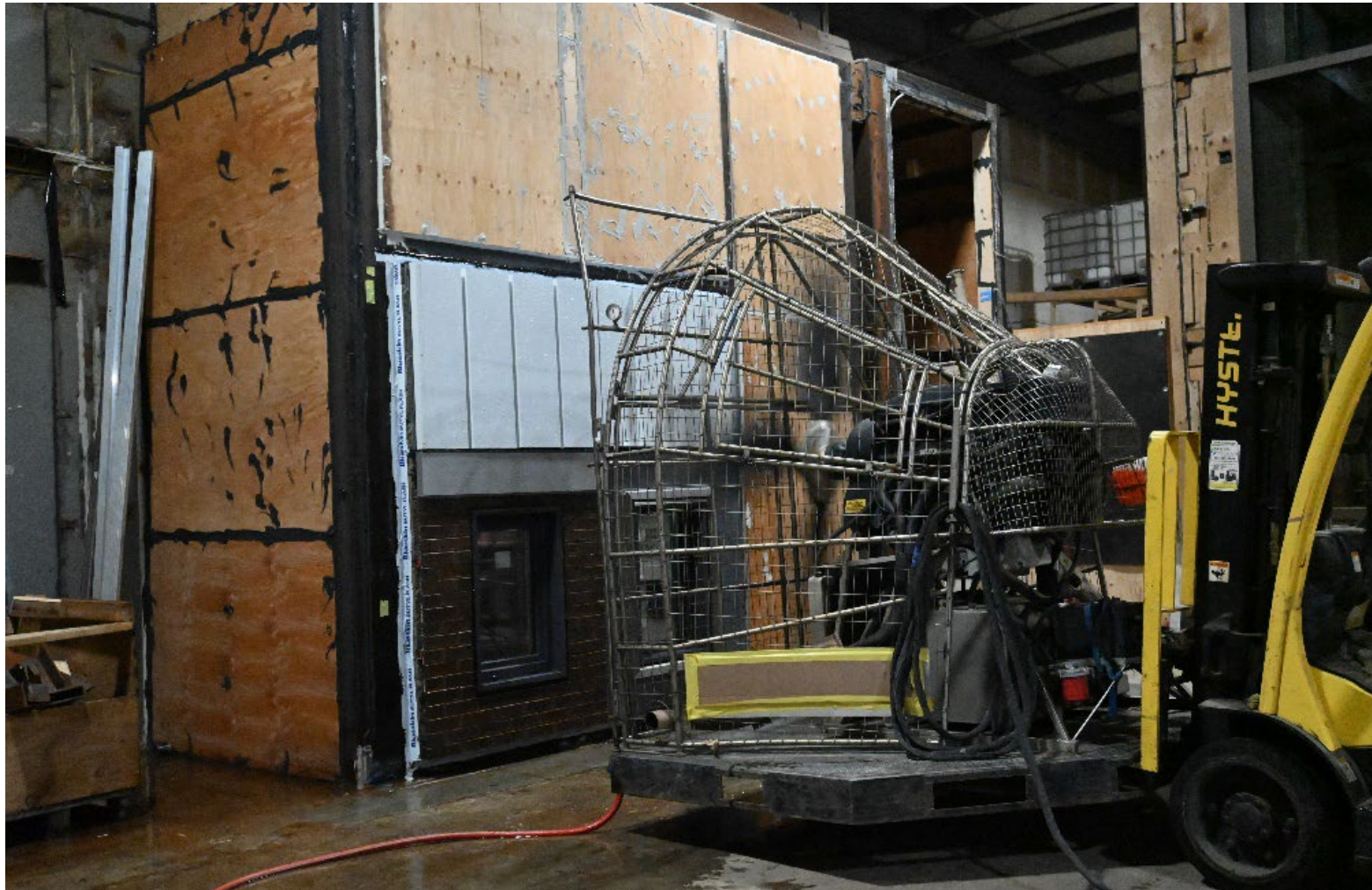
Dynamic Water Testing (AAMA 501.1)
