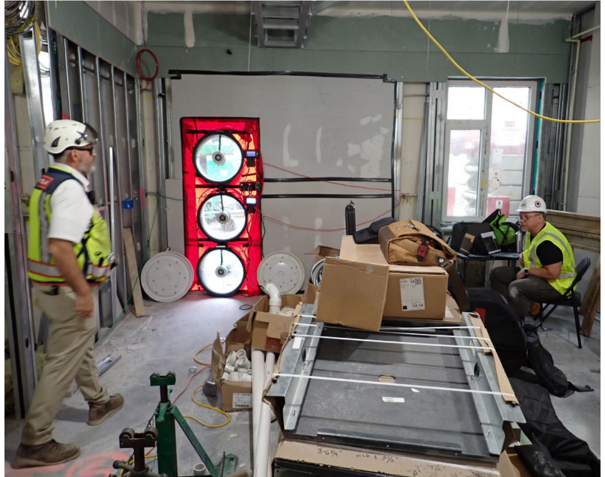
Whole Building Airtightness Testing
